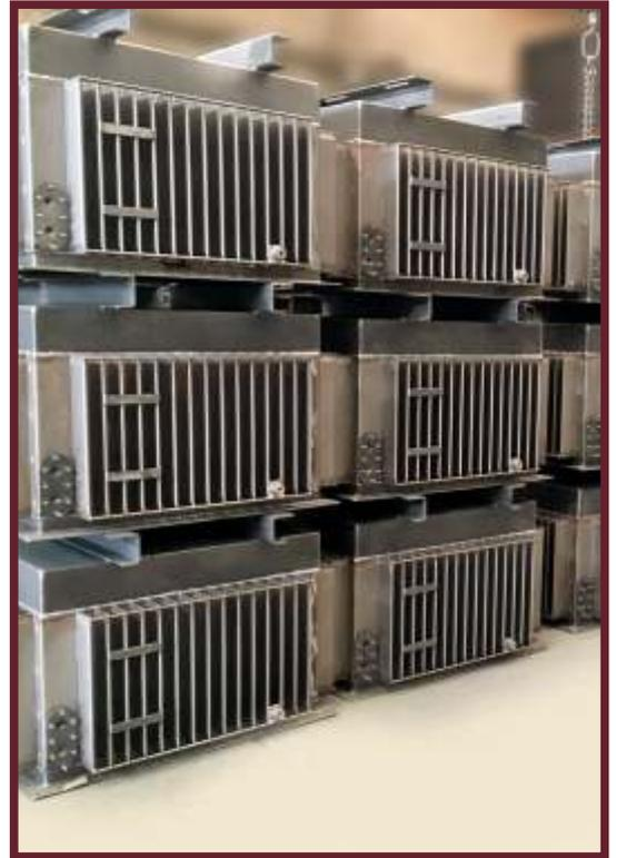
Hermetic tanks in fact need elastic corrugated wall design, while expansion tanks require more rigid design with spot-welded corrugated walls and a conservator mounted on the top.
